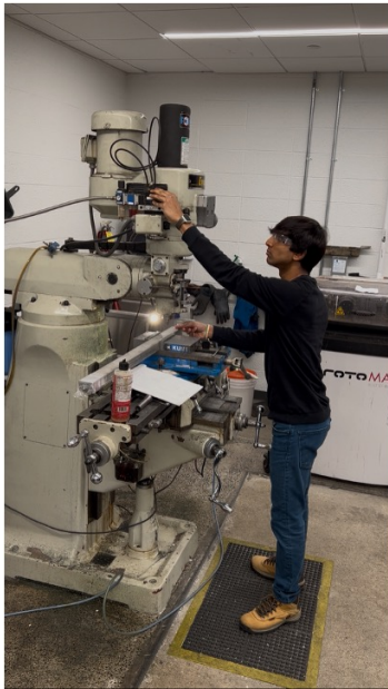
Figure 1: Machining enclosure components on the Bridgeport mill using the standardized operation-based batch workflow. 55 units manufactured on-campus.
